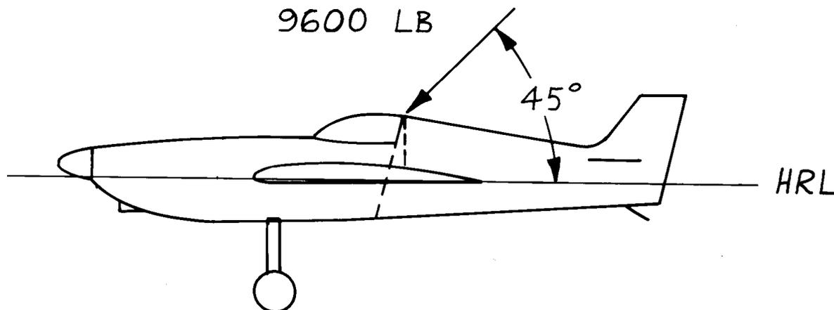
**2.6 Canopy** - It is required that the canopy be designed to have provision for unlatching from both the inside and outside in case of emergency. See Rule 11.3.
